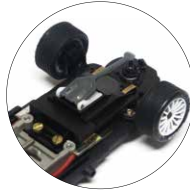
CH50 SCX digital adapter for HRS2 chassis
