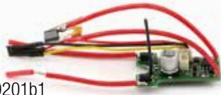
0201b1 oXigen chip in-car controller (type B)
